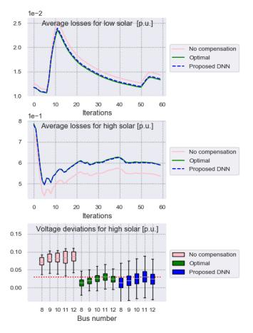
Fig. 4. Testing. Average losses for 1-2 am (top) and 2-3 pm ((middle)); voltage excursions for 2-3 pm (bottom).
