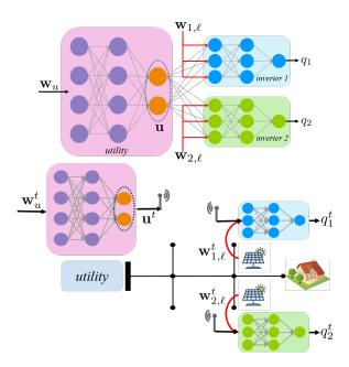
Fig. 1. Top: DNN  $\pi(\mathbf{w}; \boldsymbol{\theta})$  is organized in one utility sub-NN and inverter sub-NNs, all trained as a single DNN by the utility offline. Bottom: During real-time operation, the utility sub-NN uses real-time data to compute and broadcast the control signal, while inverter sub-NNs are run at inverters.
