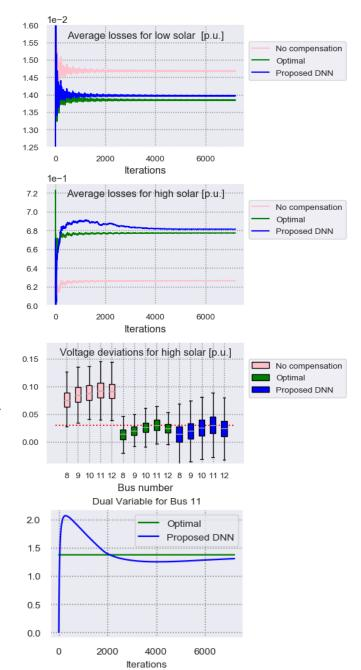
Fig. 3. Training: Average losses under no solar for 12-1 am (*top*) and high solar for 1-2 pm (*(second)*). Voltage excursions for 1-2 pm (*third*). Dual variable for active constraint on bus 11 for 1-2 pm (*bottom*).
