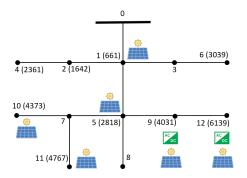
Fig. 2. The IEEE 13-bus feeder. Numbers in parentheses indicate the house index from the Pecan Street dataset mapped to each bus.
