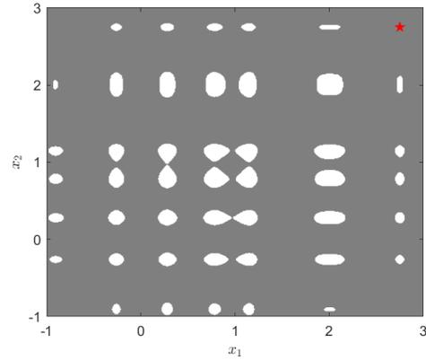
(b) Points in the grey region satisfy the proximal-PL inequality for the function  $f$  over the set  $\mathbb{S} = [-1, 3] \times [-1, 3]$  with parameters  $\mu = 0.5$  and  $\beta = 250$ , while points in the white regions do not. The unique optimal solution  $\mathbf{x}^* = (2.75, 2.75)$  is identified by a red star.
