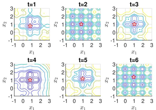
Fig. 3: Contour plots of  $f_1, \dots, f_6$  for Case A. The red star marks the unique global minimum of each function.
